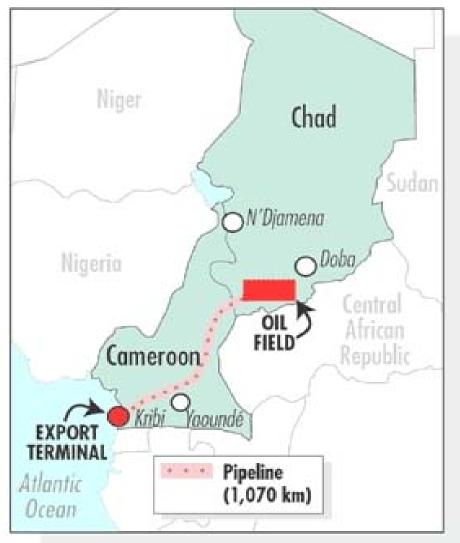
Figure 5 Planned oil pipeline from Chad to the coast in Cameroon<sup>42</sup> The length of the pipeline, finished in 2003, is 1,070 km, whereby 890 km run through Cameroon, and just 180 km through Chad. The pipeline starts at an oil field in Kome and delivers the oil to the Atlantic Coast in Kribi, where the oil can be shipped.
