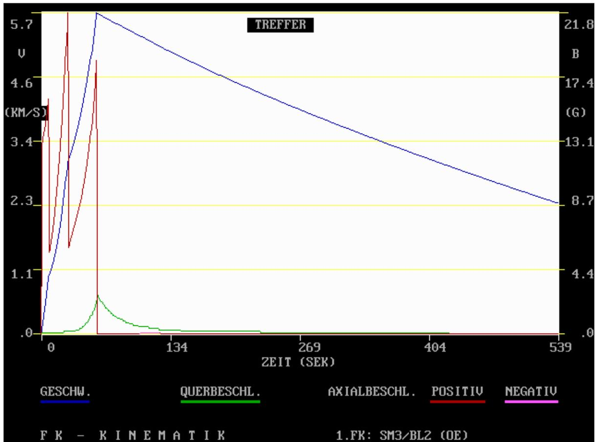
Figure 5: Kinematic parameters of the SM3-Block2 as a function of time for the interception of an R14 (OE) attack from Tehran, Iran, on Athens, Greece. The SM3 firing position is situated at Incirlik, Turkey. In this launch scenario, Phase 2 of Booster Stage 3 is ignited immediately after the burn out of Phase 1. The three axial acceleration phases of the 3 booster stages are clearly visible.
